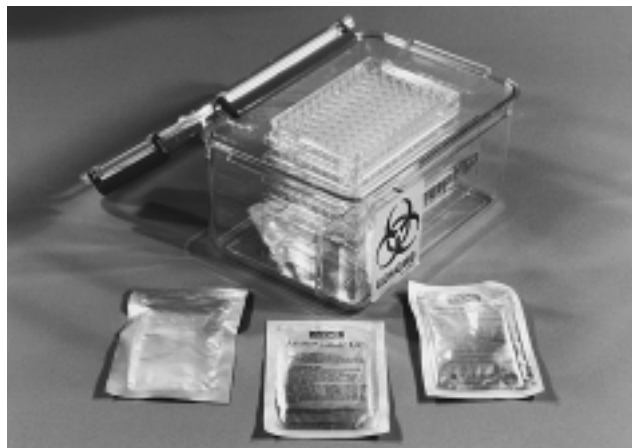
Figure 1 AneroPack sachets (from right to left: AneroPack Campylo ® , CO_2 and Plas ® ) and specific jar (AneroPack Kakugata jar ® ) with five plates.
